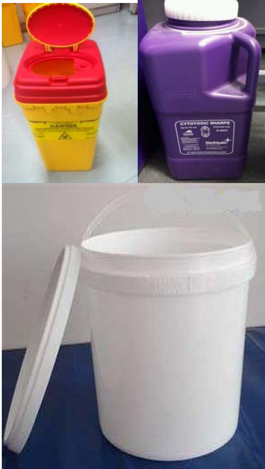
Figure 1: Sharps containers – yellow for biological, purple for cytotoxic, 20L white for broken lab glassware and larger sharps
